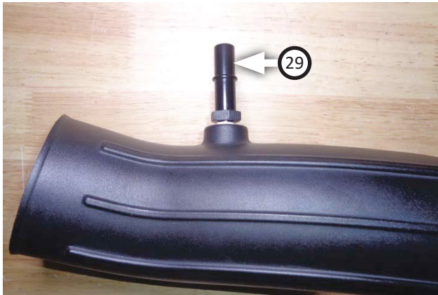
18. Apply 2 wraps of PTFE tape to quick connect fitting (29) threads then install it into intake tube.
