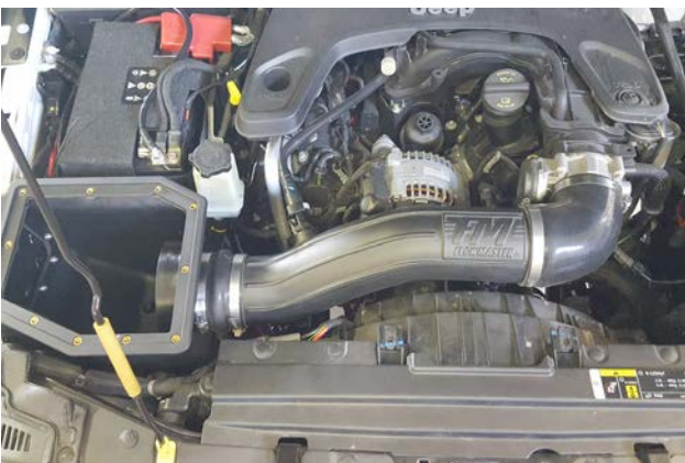
32. Set assembled intake tube into place in engine compartment and connect couplers to airbox and throttle body. Center intake tube between couplers before tightening all clamps.
