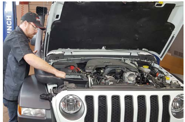
28. Place assembled airbox snorkel unit onto vehicle. Align air box into factory rubber grommets so it sets down in place.
