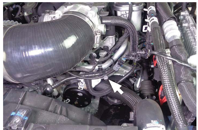
35. Use zip ties to secure temp sensor lead to nearby wiring or plumbing. Tighten all fasteners in bracket 2, 3 and snorkel completely.
