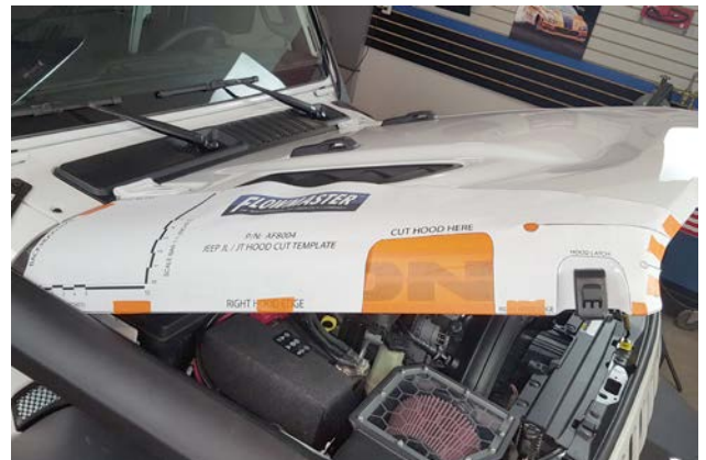
41. Fold template back onto hood and after re-aligning it, tape it down. Tape front portion down one piece at a time as shown.
