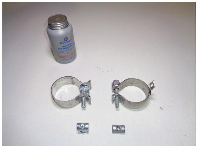
6. Fit **left (1)** and **right (2)** inlet pipes together and secure them using **clamp (9)**. Install assembly to catalytic converters with (x4 ea.) bolts and nuts (removed step 4).
